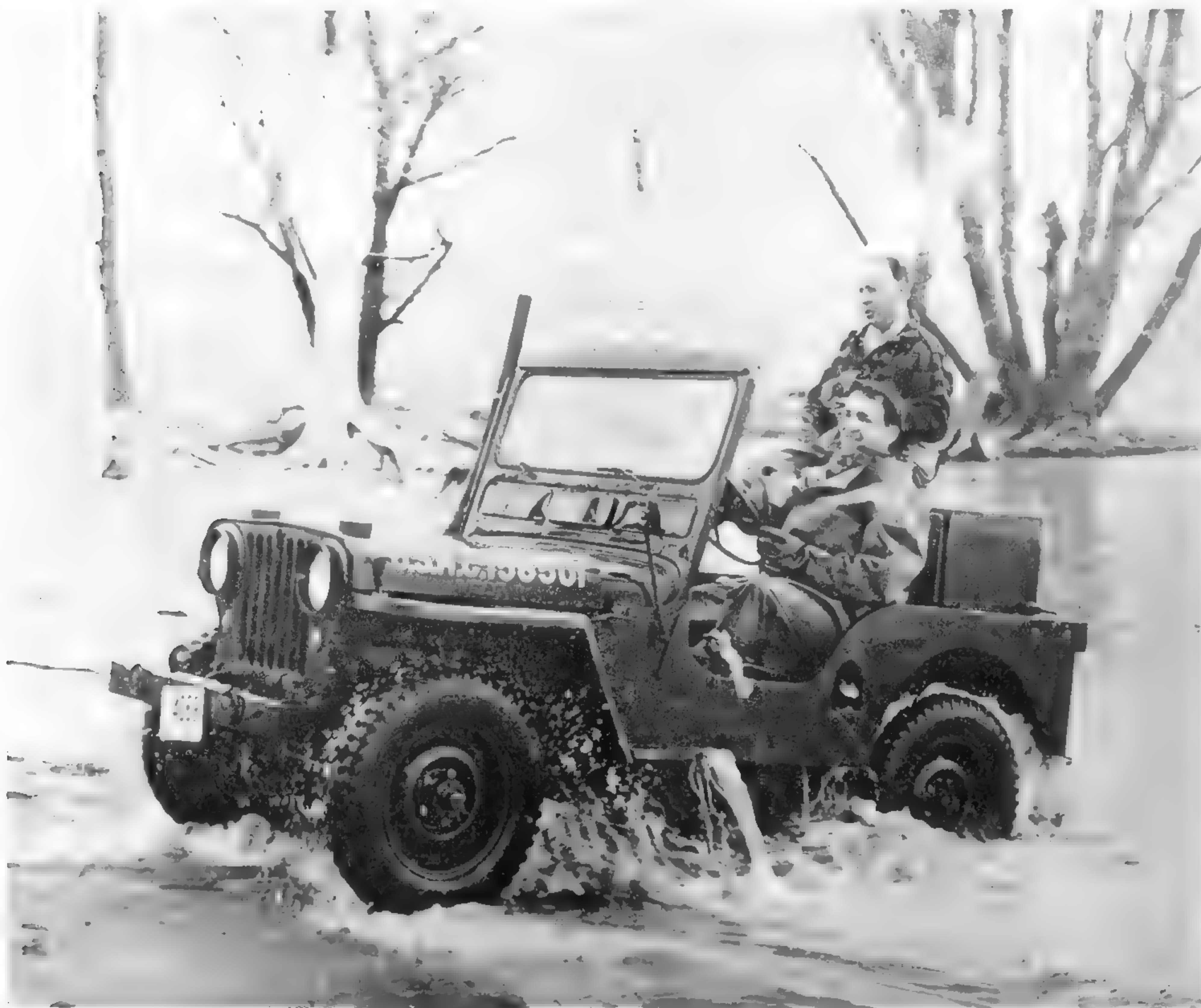
Here is the production pilot for the CJ-V35/U emerging from a fording test. The Willys name is embossed in the side of the hood. While characteristic of this model, is not correct for any other model of U.S. military Jeep. (Photo courtesy of Richard Grace collection)
